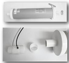
Connect flow sensor, adapter and syringe like shown in the right picture. Start the volume calibration program and start calibration procedure. Pump minimum 5 times the full volume by pumping from stop to stop.
