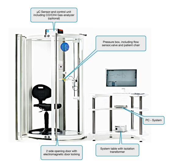
The measuring device consists of a pressure-tight chamber for the patient. On top of the chamber the electronics unit is located, it contains the signal sensors and the data acquisition unit (micro controller, sensor and control unit) with USB-interface.
