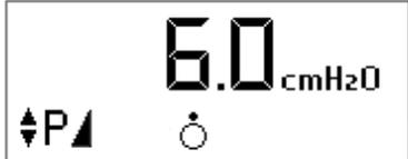
**Comfort pressure** (level of pressure produced by the device when the ramp function starts up).
