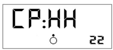
**Pneumatic Calibration** selected by your home care provider: 22 (tubing 22 mm diameter, standard), 15 (tubing 15 mm diameter), HH (humidifier), SP (specific calibration present) or -- (specific calibration absent).
