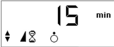
**Ramp time** (time the device takes to reach the prescribed pressure when starting from the comfort pressure when the time ramp is selected, otherwise this parameter is not displayed).
