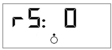
**RS232 connection selection for an external module** (a modem for example) ; it can be enabled (1) or disabled (0) by your home care provider.
